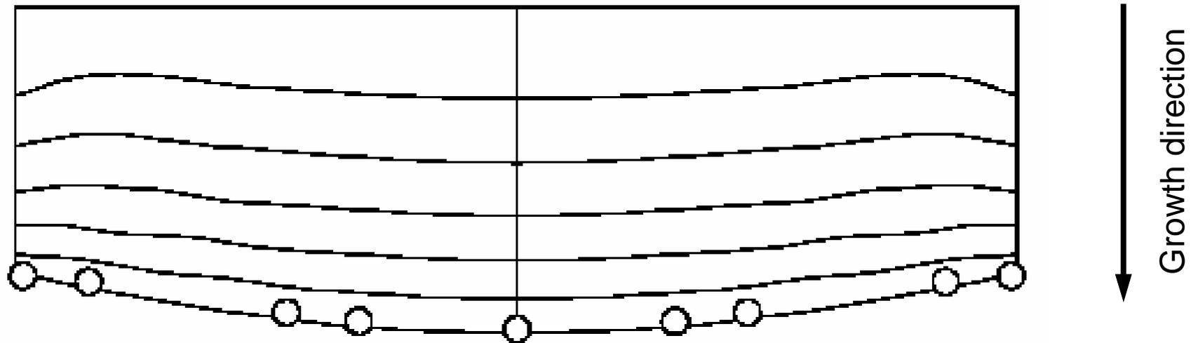
SiC boule evolution. The growth front shape is shown with an interval of 10 h
