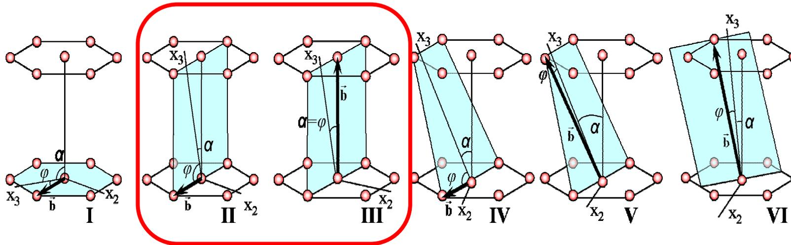
**Virtual Reactor** predicts propagation of dislocations of **II** (prismatic) and of **III** (screw) type frequently observed in the growing bulk crystal. The energetic approach was verified for modeling of dislocation behavior in thin layers and extended later for simulation of dislocation dynamics in bulk crystal growth.
