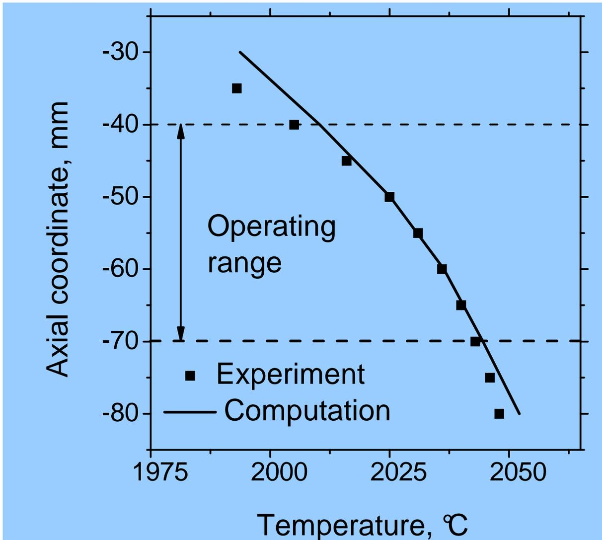
Temperature at the center of the crucible lid vs. its location at the vertical axis – comparison of the results of computations with ViR-PVT AlN™ and pyrometric measurements
