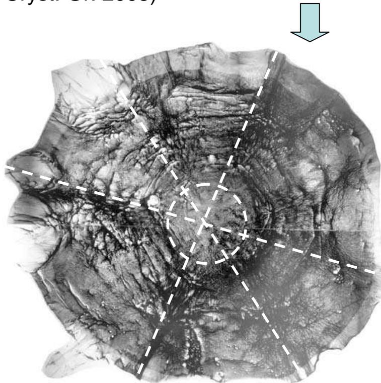
**Predicted distribution of  $\{10\bar{1}0\} \langle \bar{1}2\bar{1}0 \rangle$  TDs over the wafer surface**
