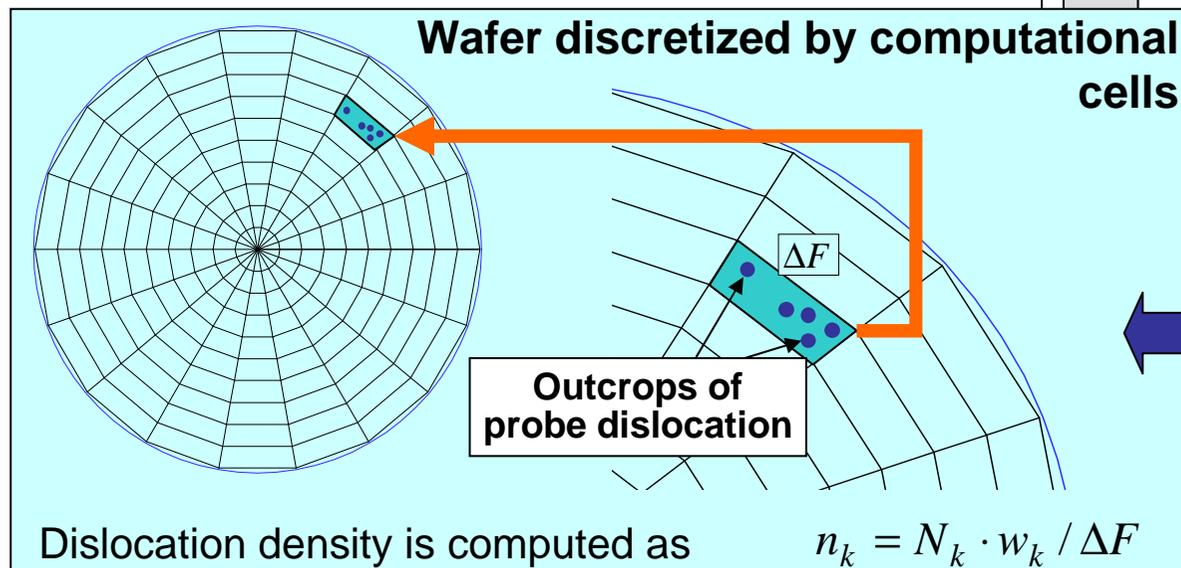
(ii) Virtual mapping, predicting the TD distribution in wafers cut from the crystal
