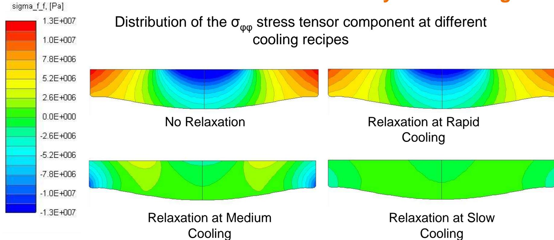
High positive values of the  $\sigma_{\phi\phi}$  stress tensor component are attributed to cause radial crystal cracking, so control of  $\sigma_{\phi\phi}$  is beneficial to provide high quality crystals
