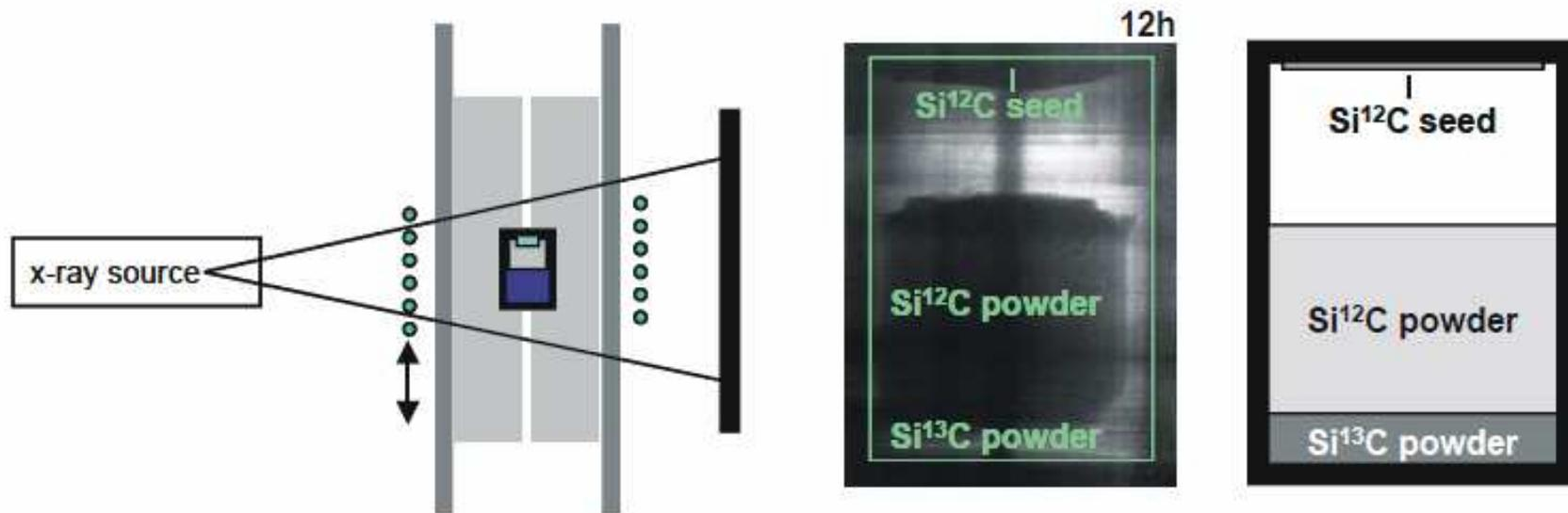
Fig. (Left) Sketch of the digital X-ray imaging setup for in situ monitoring of the SiC crystal growth process. (Center) Typical X-ray image showing the SiC crystal as well as the SiC source material with its morphology after 12 h of growth. (Right) Detailed sketch of the growth cell; in the bottom area the location of the Si<sup>13</sup>C charge for the <sup>13</sup>C-labeling experiment is pointed out.
